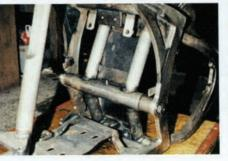
in the aluminium for tightening. To hold your forks in place a nice, neat little plug that goes in with a grub screw to hide it. First of all I thought about making half a dozen of them and every time you wanted one out, you had to drill it and stick an easy-out in it, and that was it ruined, until I eventually thought of the idea of the wee spring. So when you slacken the wee grub screw, it just pops out.
