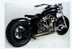
left hand side for clearance and I got special one-off exhausts made out of 1/4 wall thickness to add on the weight to the right. so it balances it out, and they weigh a ton!
